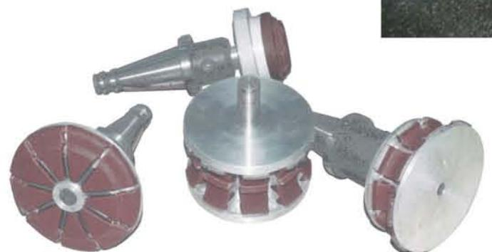
Constant diameter, which enable constant feeding speed of the pieces to be sanded (production calculation).
